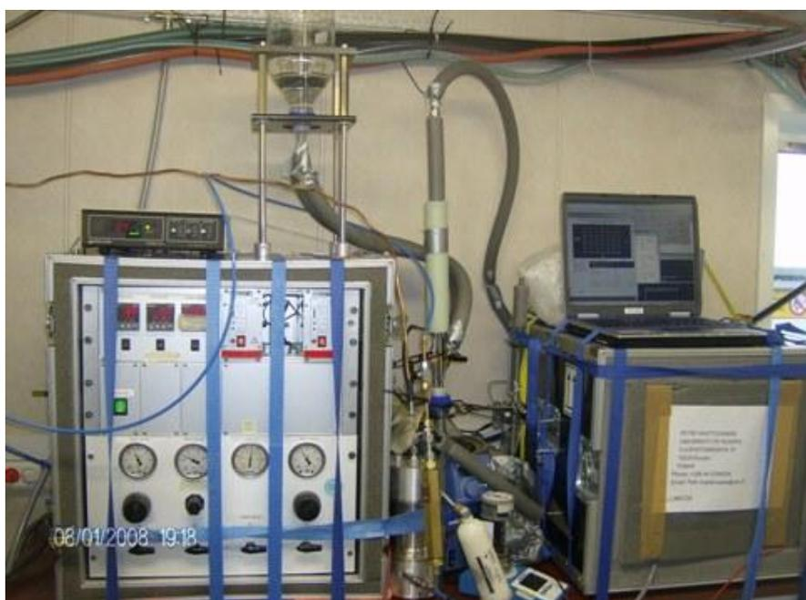
Figure 4. A ship version of the UFO-TDMA ready for an expedition.
