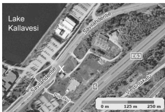
Figure 1. A layout of the Savilahti measuring site approximately 2 km from Kuopio city center between Savilahdentie road and Motorway E63. X denotes the location of the measurement site next to Savilahdentie road. Traffic flow was between 14 000 and 16 000 vehicles per weekday (Monday to Friday) corresponding to daytime traffic flow between 800–1200 vehicles h^{-1} on the Savilahdentie road.
