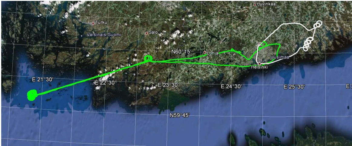
Figure 1. Flight-paths of two flights, the first flight from Vantaa (white line) only over land around town of Porvoo, the second from Vantaa (green line) over both land and Baltic Sea around Utö island. The spirals represent the vertical ascents from ~300 to ~3000 m.
