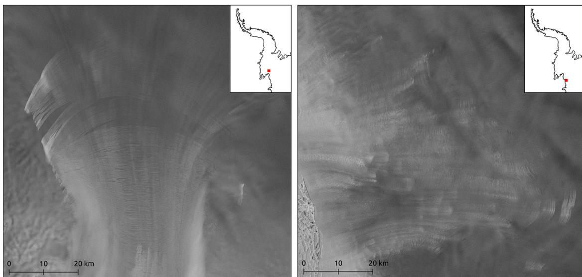
Figure 5: Crevasse upstream the grounding line of Pine Island Glacier (left) and Thwaites Glacier (right) as seen by Sentinel-1 in HH polarisation. This area of the West Antarctic Ice Sheet is projected to become instable and contains a sea level equivalent of 1.2 m, highlighting the importance of detecting change using remote sensing techniques.
