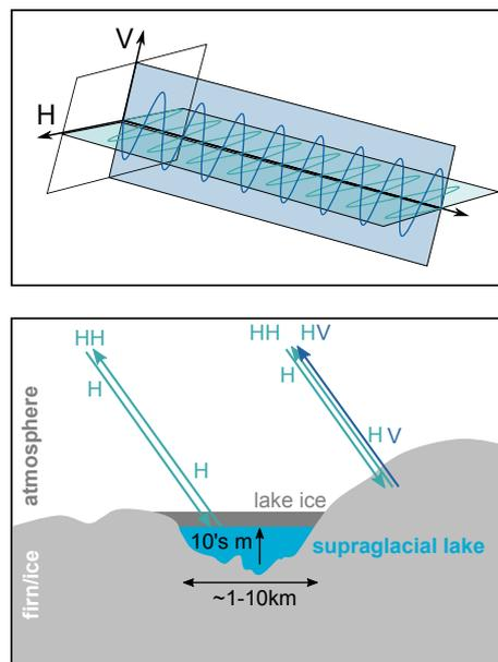
Figure 1: Top: Schematic representation of horizontal and vertical polarization. Bottom: Characteristic reflection mechanisms on an ice sheet with a supraglacial lake.
