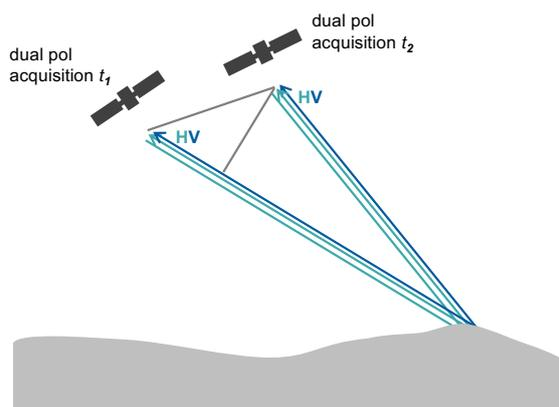
Figure 2: Schematic of the principle of PolInSAR with two different acquisitions at time  $t_1$  and  $t_2$ , recording two polarizations of the return signal each.
