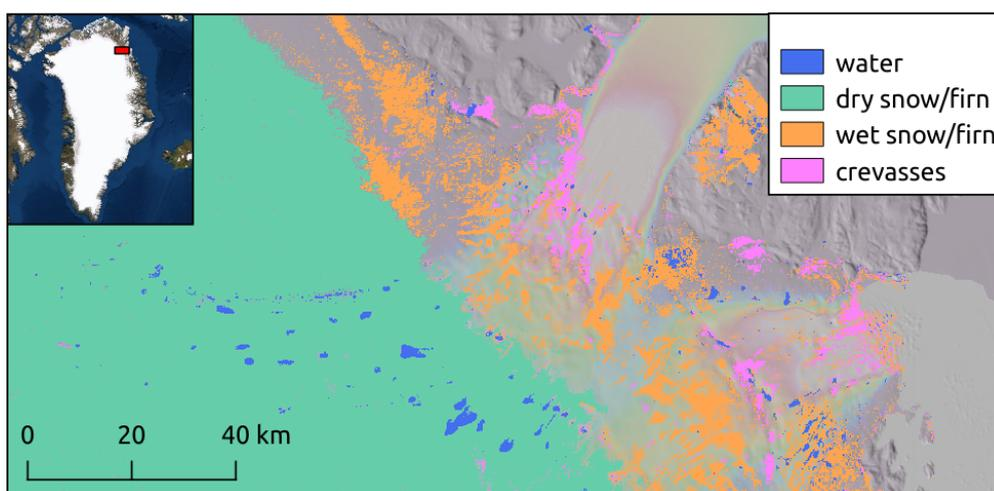
Figure 4: Example of surface types classification from a dual polarimetric Sentinel-1 scene from 2018-08-20.
