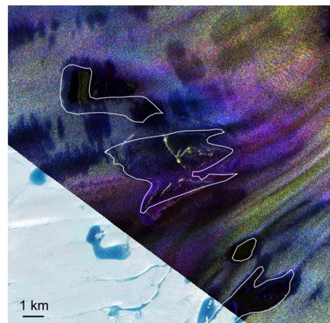
Figure 3: Pauli representation of an ALOS PALSAR image (2007-04-03) of several supraglacial lakes (white lines) at 79NG, showing  $[HH-VV]$ ,  $[HV]$  and  $[HH+VV]$  as RGB.
