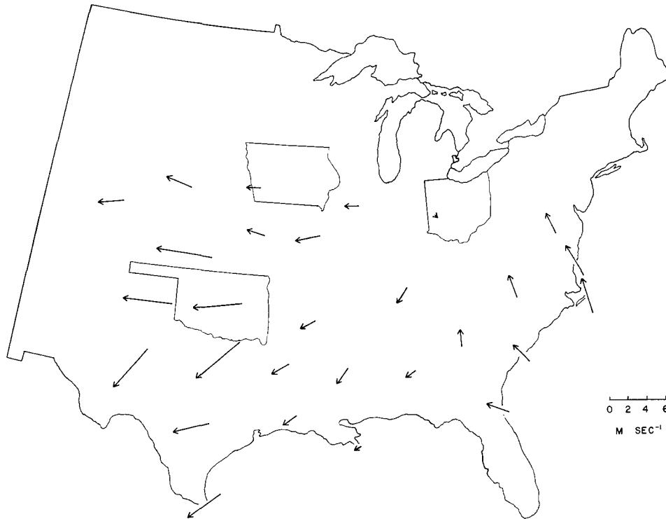
FIG. 11. 00–12 GMT mean wind difference vectors at the reporting level nearest 500 m above each station during the summer season.
