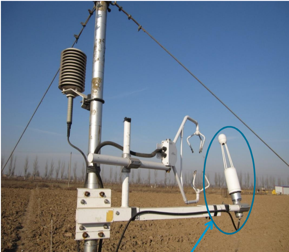
Open-path IRGA Licor 7500 ( \text{CO}_2 and \text{H}_2\text{O} )
