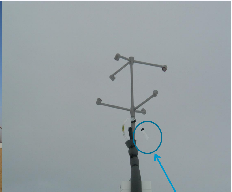
Sampling tube inlet of closed-path IRGA
