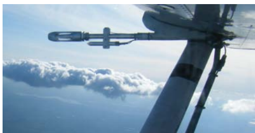
Figure 1. Photograph of the inlet mounted on the right wing during flight. The stainless steel sampling tube runs back under the wing and then along the wing strut towards the cabin where it enters from underneath. The aluminium cover tube that houses the temperature/relative humidity sensor can be seen under the inlet, with cables being passed along the sampling tube towards the inside of the airplane.
