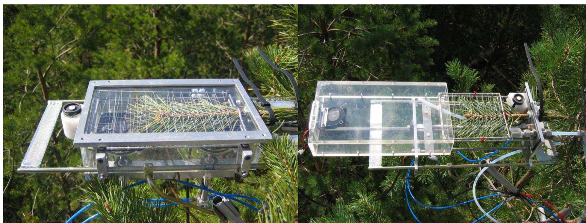
Figure 1. Left: box chamber, right: sliding chamber. Photos: Pasi Kolari
