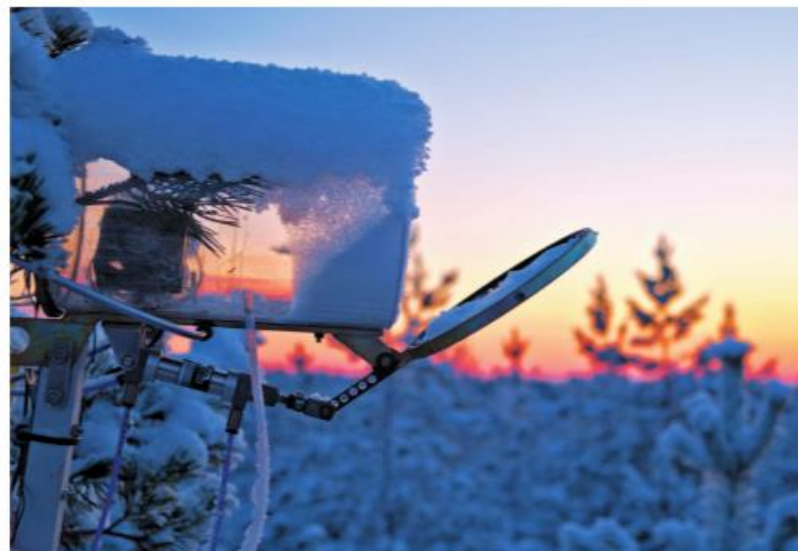
An enclosure for measuring gas exchange between plants and the atmosphere at a station in Finland.
