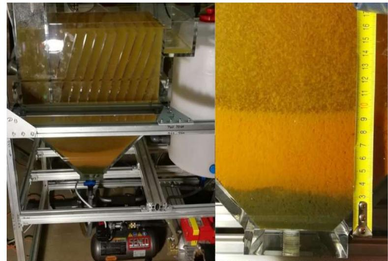
Sludge in grouped thickener after electrochemical coagulation
