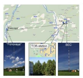
Fonovaya (56°25'N, 84°04'E): Measurements of meteorology (T, P, U, RH), Trace gases (CH<sub>4</sub>, CO<sub>2</sub>, NO, NO<sub>2</sub>, SO<sub>2</sub>, CO, O<sub>3</sub>) Aerosol measurements: Diffusion battery + CPC Optical Particle Sizer
